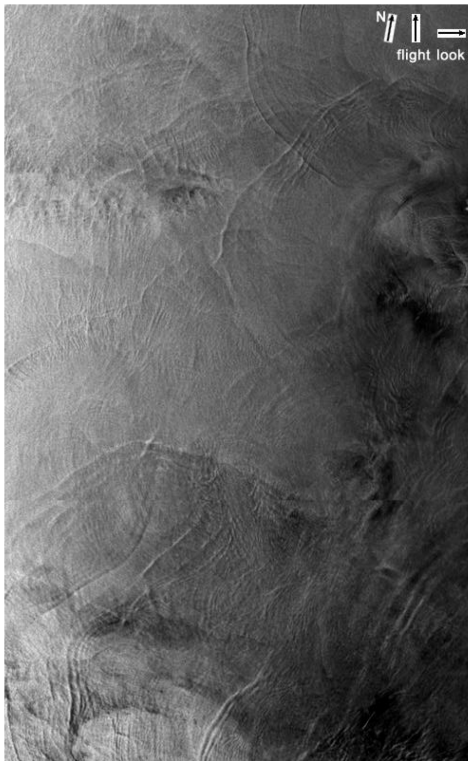
Figure 2. ERS-2 C-Band VV SAR image collected on October 1, 1998. The image shows an area north of Sakhalin Island with a number of internal wave signatures having a variety of propagation directions. This indicates there are several source locations. Image dimensions are 100 km x 140 km centered near 56^{\circ} N. latitude, 143^{\circ} E. longitude. [Image from ADI'DAS Radar Image Preview Database. http://adidas.iki.rssi.ru ]
