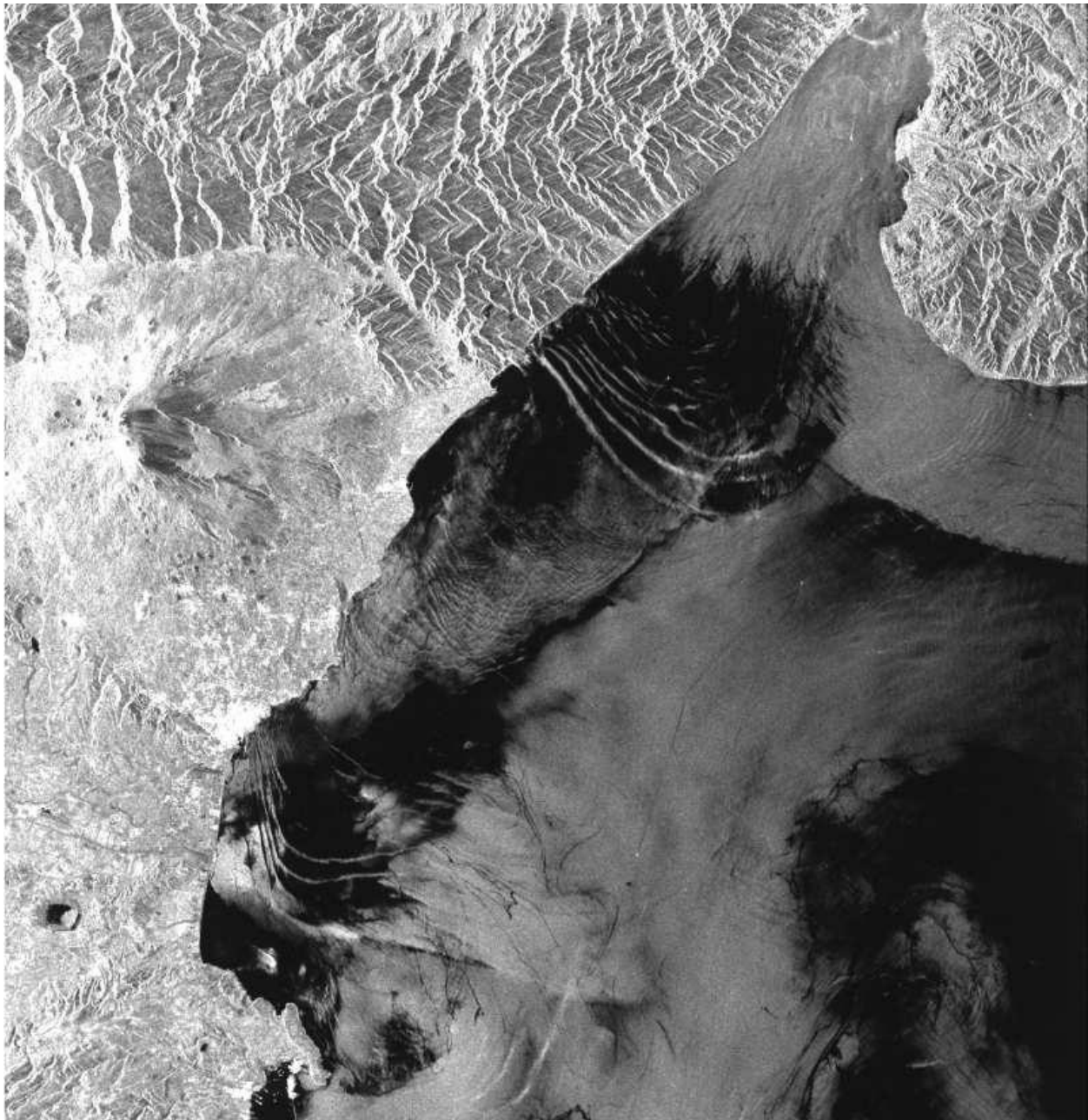
Figure 2. ERS-1 C-Band VV SAR image of the Strait of Messina collected on September 22, 1994 at 21:15 GMT (Orbit: 16672, Frames: 0747). Image dimensions are 100 km x 100 km centered at 37°38' N. 15°22' E. The image shows signatures of two prominent internal wave packets propagating south out of the strait with the signature of a smaller, less intense packet between them. [ERS-1 image ©ESA 1994, from The Tropical and Subtropical Ocean Viewed by ERS SAR http://www.ifm.uni-hamburg.de/ers-sar/ ]
